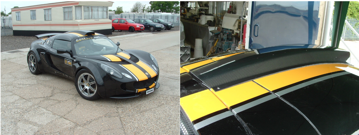
Gt3 Exige S2 Cadena sport replica shown with larger carbon intercooler scoop (bolt on)
